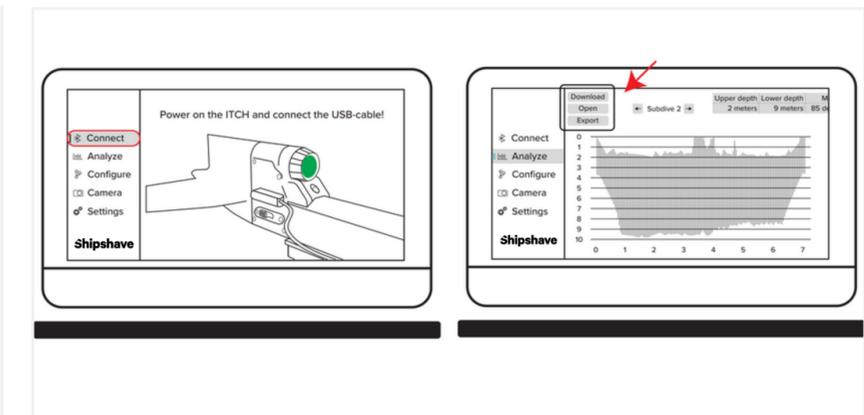
8. Transfer data and video using Slick. Assess hull condition and repeat the operation if necessary.
