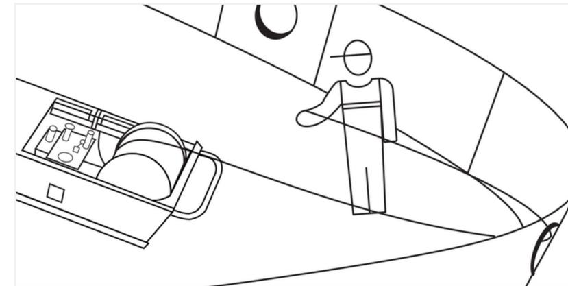
3. Lead rope out center fairlead using shive on outside. Bring it back onto deck; tie to the robot with bowline knot.
