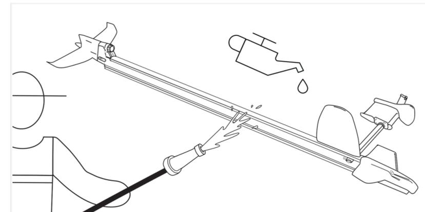
7. Rinse robot and winch using fresh water. Check for wear. Spray robot with penetrating oil.
