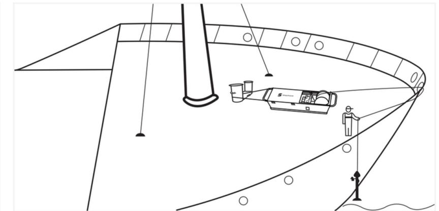
4. Power on, confirm solid green light. Lower robot on correct side.
