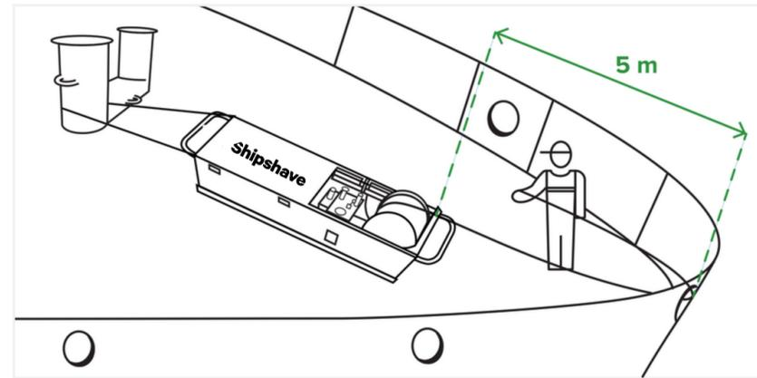
2. Secure the winch and connect power. Inspect and cut worn rope.
